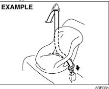
Install your child restraint system according to the instructions provided by the child restraint system manufacturer. If you install the child restraint system in the front seat, be sure to slide the seat to the rearmost position. After making sure that the seat belt is securely latched:
